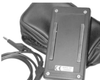
Photo at left shows contact rails on base of instrument. To measure surface resistivity of a flat sample of material simply place the instrument on the material so that these rails are in contact with the
